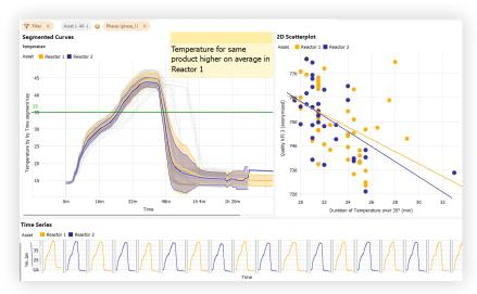
Comparing batch profile curves across two reactors reveals different temperature levels for making the same product, indicating optimization potential.
